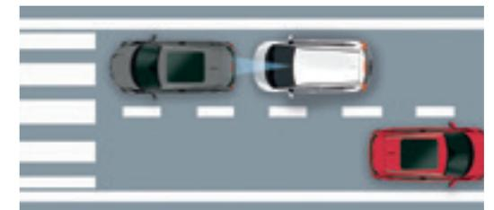
**3:** If you've still not reacted, and a collision is imminent, the City-Brake Active System can automatically apply emergency braking to reduce speed as much as possible. In good driving conditions, it could even avoid a collision altogether.
